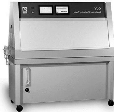
6. QUV Accelerated Weathering Tester
