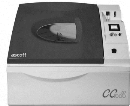
8. Salt Spray Test Chamber
